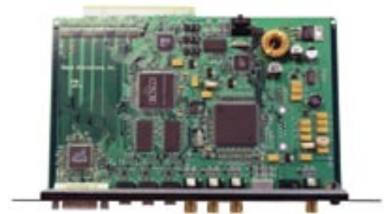
All Vivix™ processing is located on a modular controller card.
